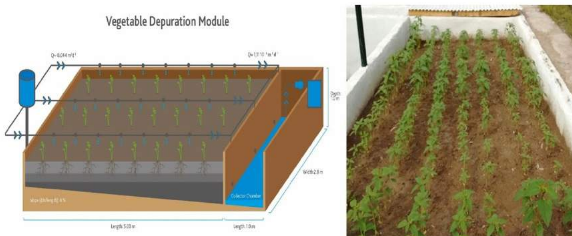
Figure 3. Diagram of the Vegetable Depuration Module and the phyto-mycoremediation system ( Helianthus annuus – Rhizophagus intraradices ) with 2 m 3 volume and 20 plants per m 2 (Scotti et al., 2019).
