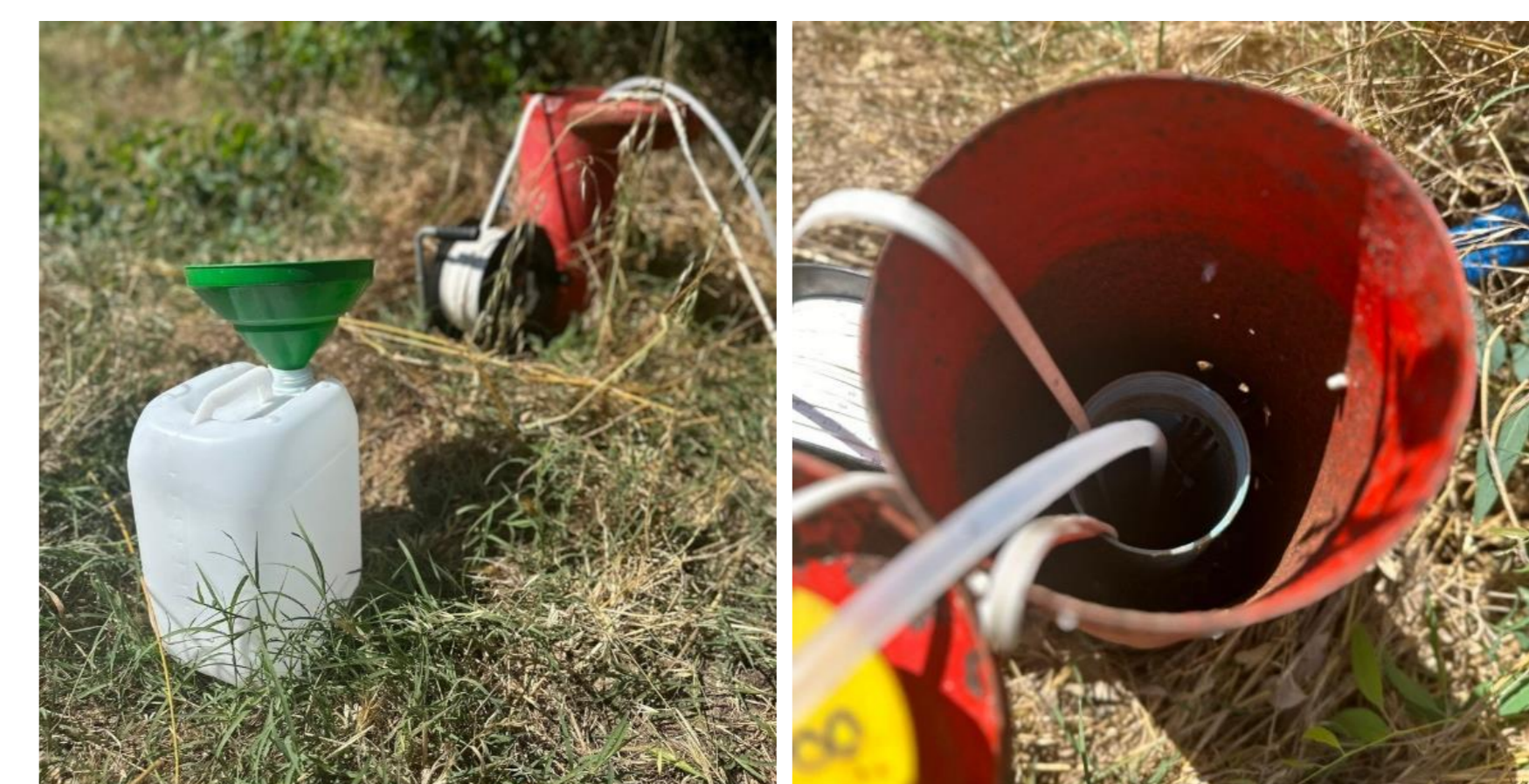
Figure 3. Sampling groundwater from the Arborea zone
